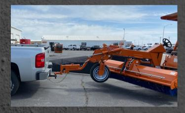
The BB250 comes with a standard hydraulic tow hitch that lifts the front wheel and enables the machine to be towed on only its back two wheels for maximum stability.
