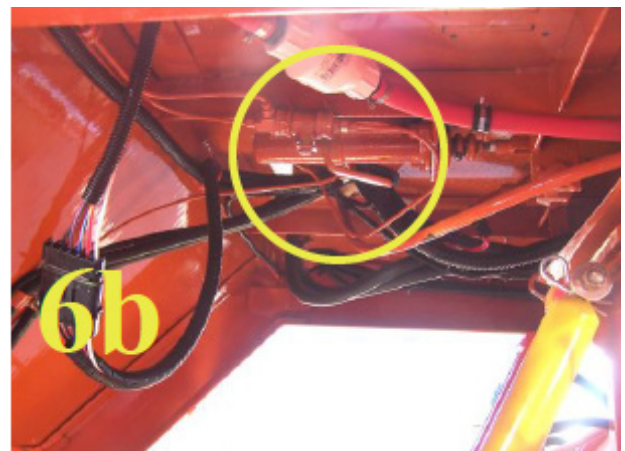
Surge brake only - close valve for towing (valve open in photo)
