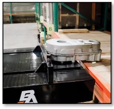
To remove, unsecure the die from the drawbar. Use the drawbar to push the die off the platform and into its new spot.
