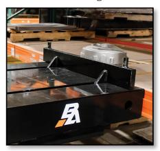
As you approach the die, align the drawbar with the center of the die. Secure your die to the drawbar.
