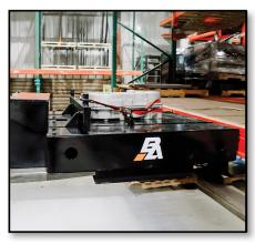
Engage the hydraulic motor to drive the drawbar back, pulling the die onto the platform. Transport your die to its designated spot.
